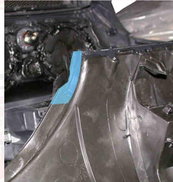
Close the ventilation duct inlet using a made-to-measure aluminium or plastic plate. Seal the whole rim with a silicon seal.
