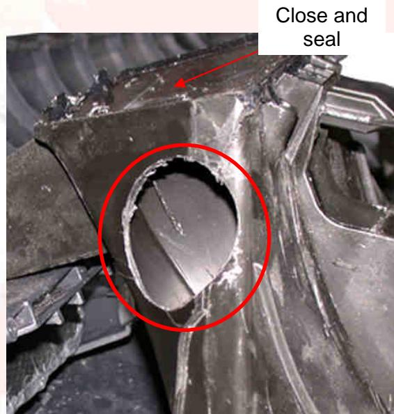
Glue the right and left defrosting connections (ref.3) on the duct, as shown in the photo opposite.
