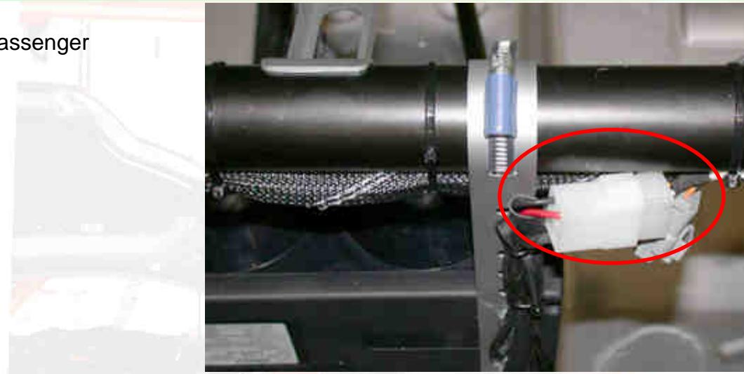
Wedge the heating unit with a block of foam, cut beforehand to follow the shape of the turbine (see photo opposite).
