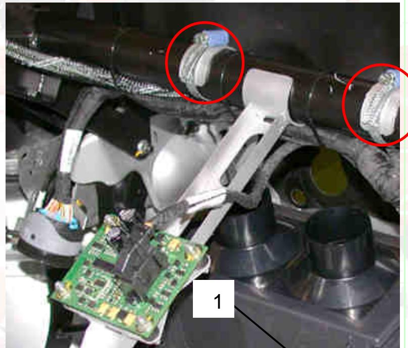
Connect the heating unit on the passenger compartment bundle.
