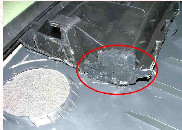
Cut the dashboard for the passage of the arch, driver's and co-driver's side.
